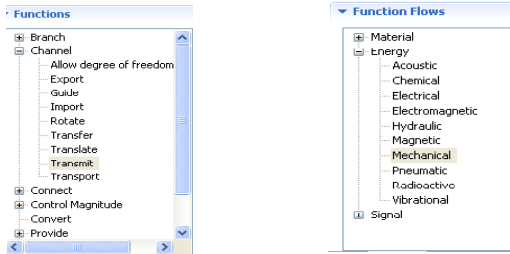
Fig. 4. Selection of functions and flows for a drive shaft
