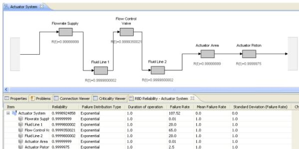
Figure 4 – Reliability Block Diagram of the system
