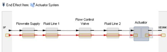
Figure 1 – Functional model of Actuator System
