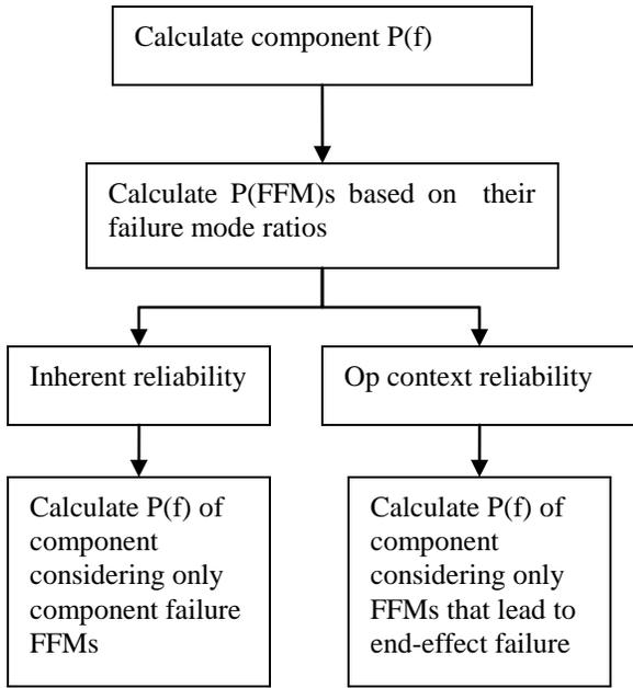
**Figure 7 - Flowchart for component reliability calculations**
