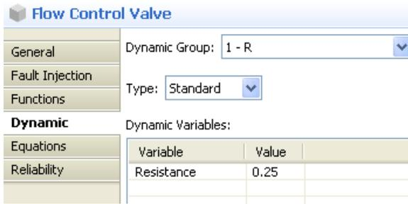
Figure 3 –Dynamic properties of the Flow Control Valve
