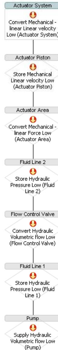
Figure 5 – Fault Tree display of a cut set for actuator system failure.
